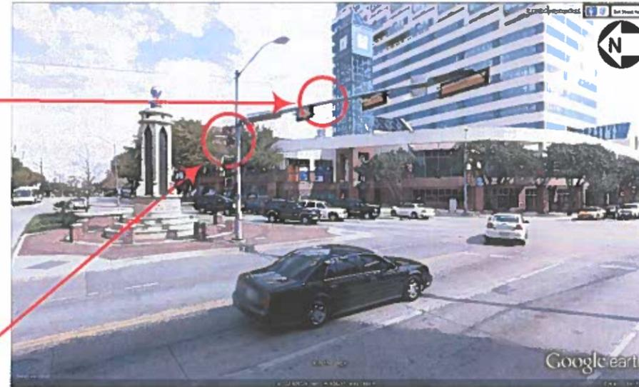
Install equipment enclosure here with cover facing northeast.
